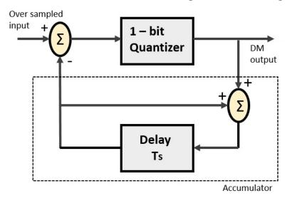
A stair-case approximated waveform will be the output of the delta modulator with the step-size as delta ( $\Delta$ ). The output quality of the waveform is moderate.
