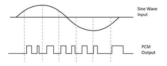
Instead of a pulse train, PCM produces a series of numbers or digits, and hence this process is called as **digital**. Each one of these digits, though in binary code, represent the approximate amplitude of the signal sample at that instant. In Pulse Code Modulation, the message signal is represented by a sequence of coded pulses. This message signal is achieved by representing the signal in discrete form in both time and amplitude.
