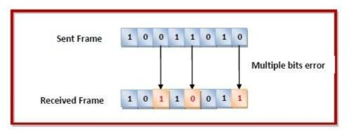
Burst error – In the received frame, more than one consecutive bits are corrupted.
